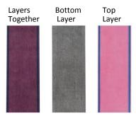
8387 offers a unique multi colored construction, making it more visible to remove the splice during converting
