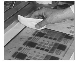
polymer plate making process. This residue can lead to plate lifting and must be removed prior to mounting plates. Wash using an Isopropyl alcohol solution to remove this photopolymer residue.
