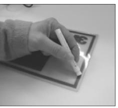
inner vial and release the adhesion promoter. Slightly squeeze to allow for liquid to wet the tip of the ampule. Apply to the lead and trail edge of the photopolymer plate. Use a minimum amount to wet the surface. More is not better.
