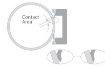
**THE INCORRECT PRESSURE** Or excessive blade pressure creates free floating metal slivers that contaminate ink systems. When a hard particle becomes trapped between the deflected blade tip and the anilox, this particle rides there, effectively destroying rows of cells. These rows of cells appear as thin bands running the circumference of an anilox and are commonly called score lines.
