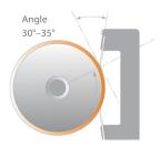
**CHAMBER DOCTOR BLADE SYSTEMS** There are two distinctly different blade systems; single Reverse-Angle Blade system and the more commonly used Enclosed Doctor Blade System. Angles on an enclosed system are pre-set and for single reverse-angle blade system the industry standard is approximately 30 to 35 degrees. Flat angles create greater contact area, requiring more doctor blade pressure to get a clean wipe. This increase in pressure creates excessive anilox and blade wear.
