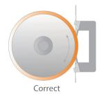
**PROPER SYSTEM ALIGNMENT** For consistent ink metering, best print quality and optimized blade life, an enclosed chamber system requires perfect alignment (both horizontal and vertical) so that both blades have equal amounts of pressure. Incorrect alignment creates uneven blade pressure, blade wear and/or ink leakage.
