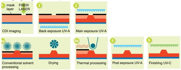
The digital flexo plate has a mask layer – sensitized to the CDI's laser light – on top of its surface. After imaging, this mask takes the function of the traditional film negative. Through the integration of the image carrier, a digital flexo plate has sharper image definition and steeper relief shoulders than conventional plates produced with film. Image deterioration by UV light absorption and scattering in the traditional contacting through vacuum sheet and film is totally eliminated.
