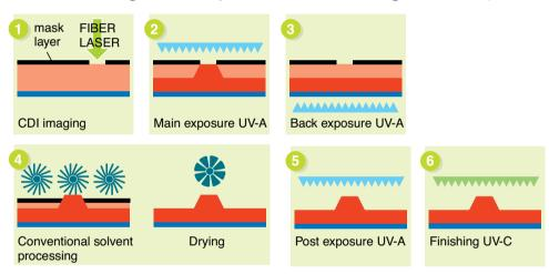
The digital flexo plate has a mask layer – sensitized to the CDI's laser light – on top of its surface. After imaging, this mask takes the function of the traditional film negative. Through the integration of the image carrier, a digital flexo plate has sharper image definition and steeper relief shoulders than conventional plates produced with film. Image deterioration by UV light absorption and scattering in the traditional contacting through vacuum sheet and film is totally eliminated.
