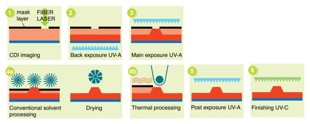
The digital flexo plate has a mask layer – sensitized to the CDI's laser light – on top of its surface. After imaging, this mask takes the function of the traditional film negative. Through the integration of the image carrier, a digital flexo plate has sharper image definition and steeper relief shoulders than conventional plates produced with film. Image deterioration by UV light absorption and scattering in the traditional contacting through vacuum sheet and film is totally eliminated.
