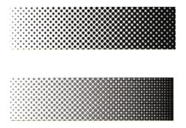
When jobs are ready for final output, the true PDF 1.7 native RIP optionally available in Odystar outputs color data to proofing equipment as well as screened information to plate. Advanced screening technologies include Paragon, Organic and Concentric Screening, which combines the smoothness of AM with the advantages of FM: higher saturation, better quality, more detail and important ink savings.
