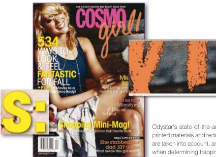
Odystar's state-of-the-art trapping tool allows for better quality printed materials and reduction of paper waste. All transparencies are taken into account, and even the image content is considered when determining trapping directions. Trapping simply becomes an automated step in the process of making the job print-ready. And as the trapping is object-based, traps can be previewed and even edited in native PDF editing tools like Neo.
