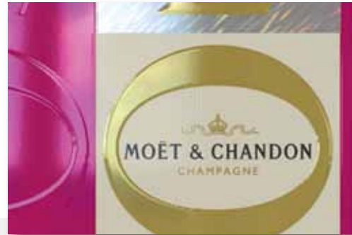
Visualizer print modeling of a foil board overprinted with black, pink and yellow, an opaque white, a holographic hot stamp foil, micro embossing and rounded embossing.
