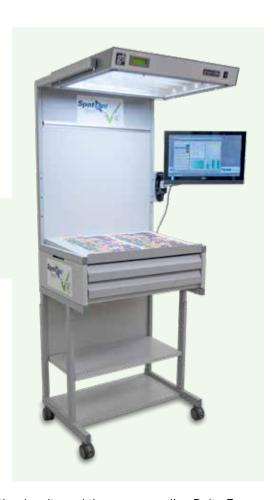
The SpotOn Color software also provides a trending chart of the density and the corresponding Delta E versus the reference color during the press run and a reporting function that summarizes the press run.
