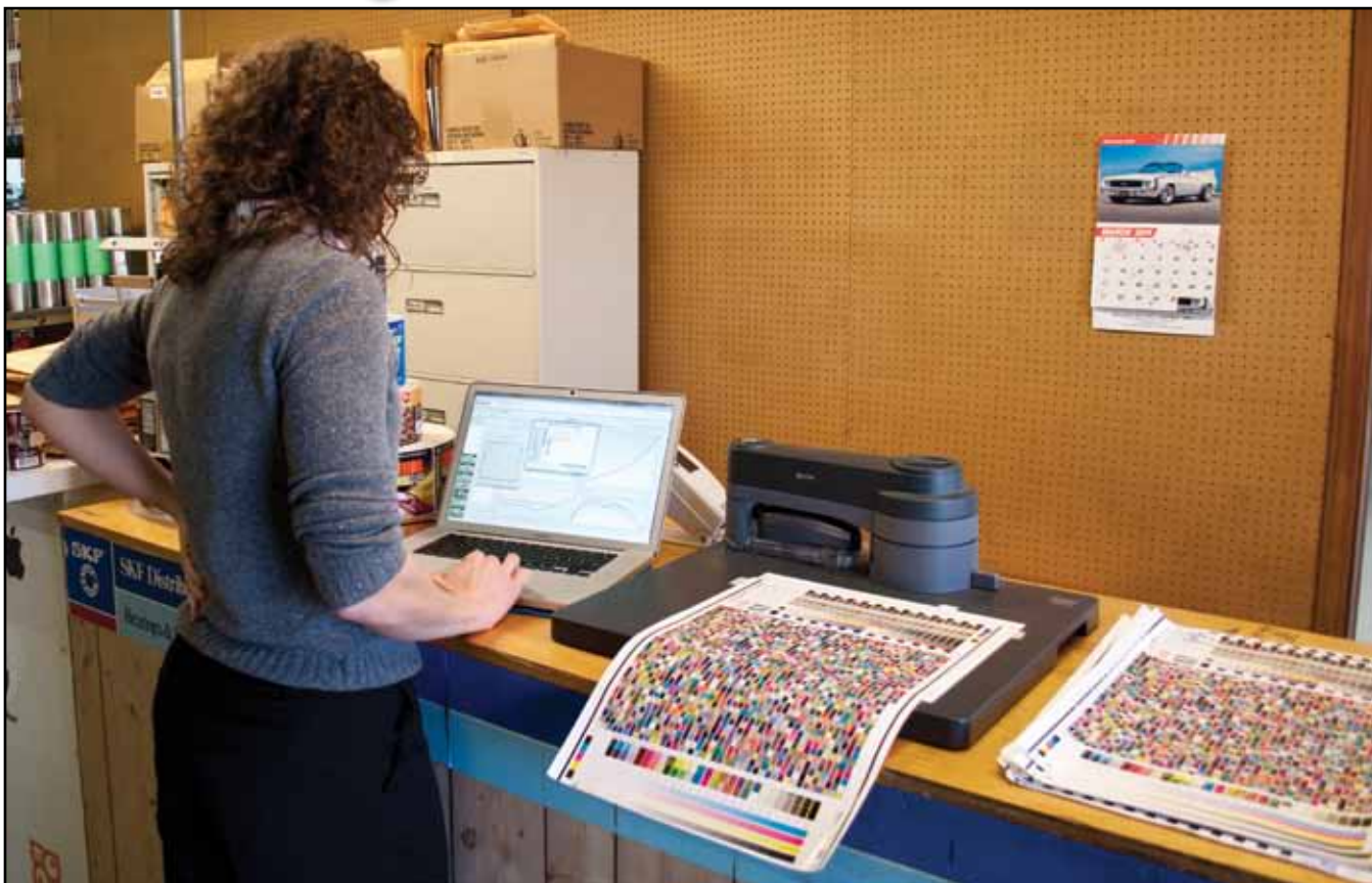
The author takes measurements with a spectrophotometer, then documents results, using all-important control targets.
