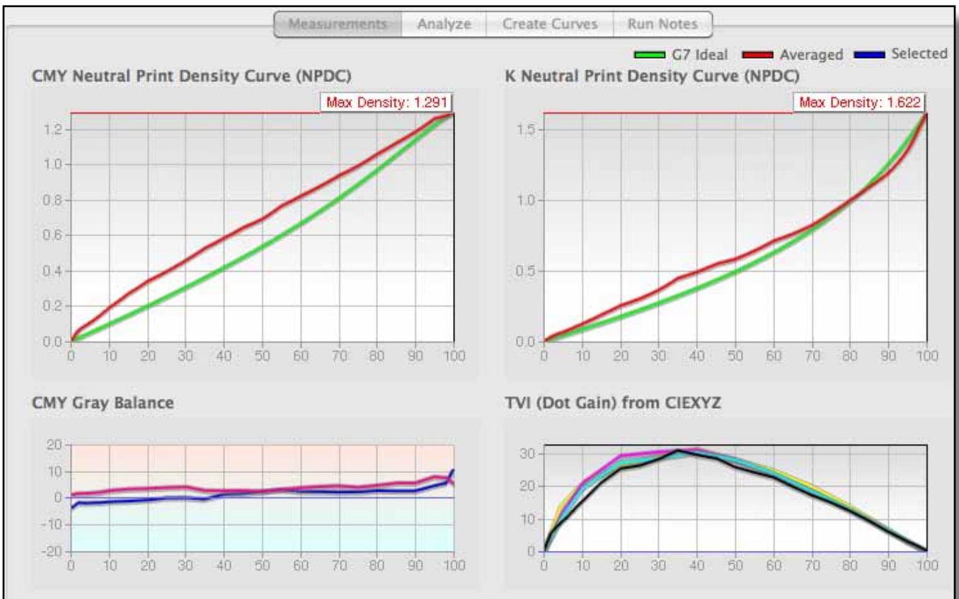
FIGURE 1. Screen capture of IDEAlliance Curve2 software analysis of the linear P2P target. The NPDC curve is based on measurements from several print samples and is slightly higher than the target NPDC curve. However, the CMY gray-balance curves indicate their process has a natural gray balance.
